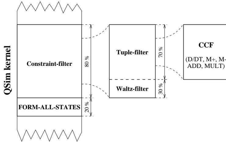
**Fig. 1.** Runtime analysis of the QSIM kernel. Kernel functions are hierarchically structured and their runtimes are informally presented with regard to the runtime of the calling function. The presented runtime ratios are extracted from various runtime measurements of a QSIM system implemented on a TI Explorer LISP workstation.
