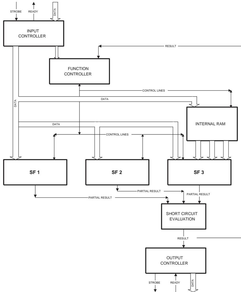
**Fig. 3.** Block diagram of the MULT-CCF coprocessor. The input and output controller connect the coprocessor to the host processor via an 8 bit data bus and two handshake lines (STROBE, READY). For simplification control lines between input/output controller and function controller are not shown.
