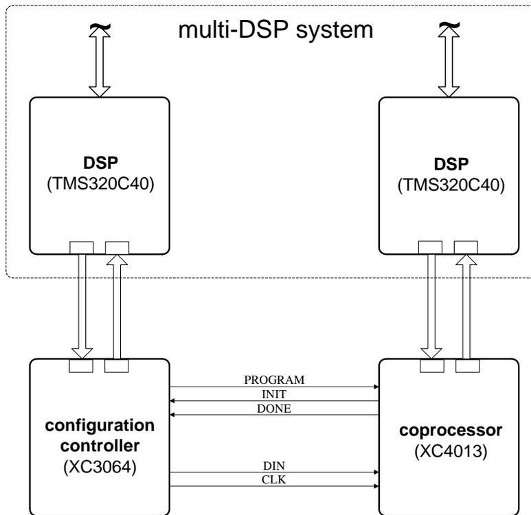
Figure 1: Block diagram of the basic architecture. The configuration controller and the coprocessor are connected to two DSPs of the multi-DSP system via two communication channels.
