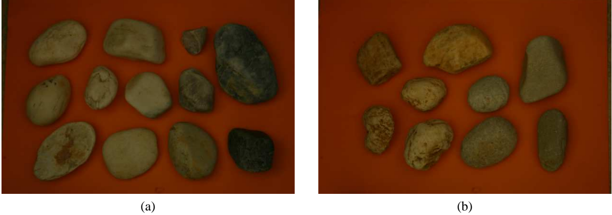
Fig. 15. Example materials for granulated material separation: (a) precious rubble (referred to class 1), and (b) worthless rubble (referred to class 2).
