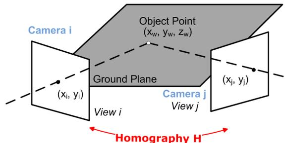
**Fig. 3.** Homography induced by a plane.
