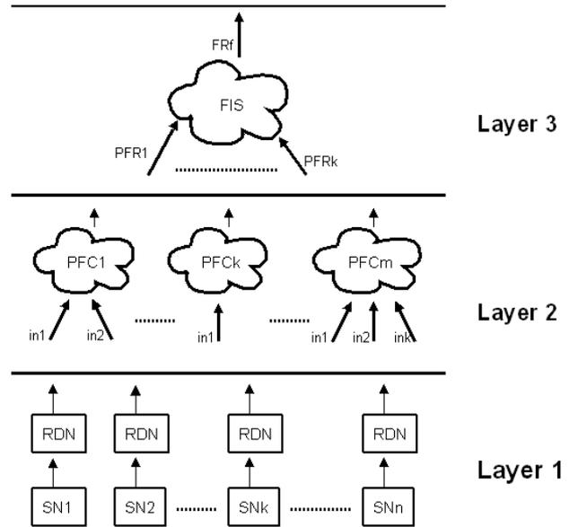
Fig. 2: Three-layered fusion architecture. Legend:  $SN_i$  (sensor node),  $RDN_i$  (raw data acquisition and normalization),  $in_i$  (observed data from layer 1),  $PFC_i$  (partial fusion clusters),  $PFR_i$  (partial fusion results), FIS (fuzzy inference system),  $FR_f$  (final decision). Explanation of the different components given in section 3.
