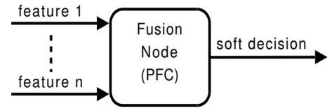
Fig. 3: Fusion process. Input features originate from homo-/heterogeneous sensors and are fused appropriately forming a soft decision.
