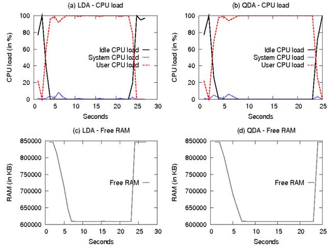
Fig. 6: LDA and QDA - CPU load and RAM usage ( $n_{ts} = 100000$ ) where CPU and RAM parameters are recorded starting approx. 2s before and stopping approx. 2s after executing the algorithms (hence the "transitions")
