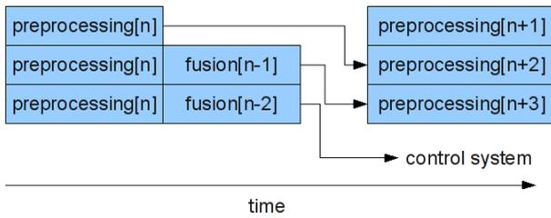
**Figure 2: Pipeline fusion approach, increased frame rate**
