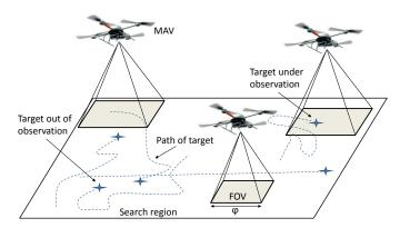
Fig. 1: Observing multiple moving targets using cooperative MAVs.
