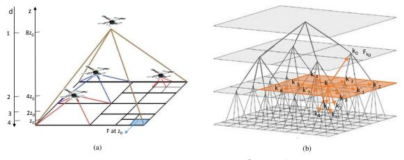
Fig. 2: Model for the MAV movement: (a) Relationship of search region  $\Omega$ , FOV (F), altitude (z), lowest altitude (z<sub>0</sub>), and depth (d) of the quad-tree. (b) Fourteen-neighborhood (orange arrows and square around the current node k).
