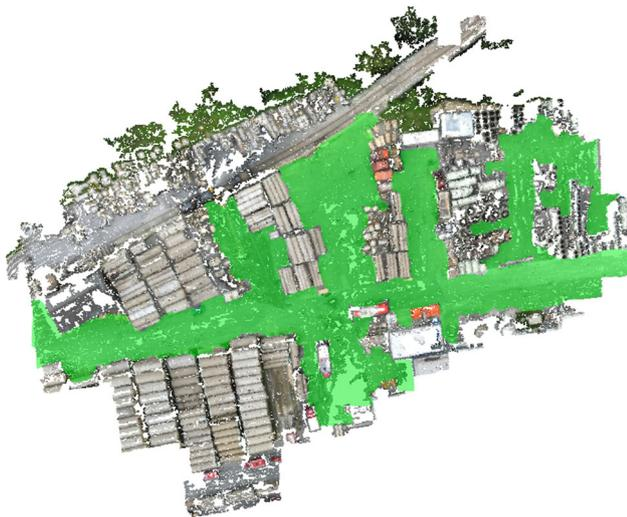
**Fig. 11** In this dense point cloud (enhanced by patch-based multi-view stereo method (PMVS) [17]) the observed area is presented from nadir view and the ground plane is manually annotated in green. This plane is our request projection plane (color figure online)
