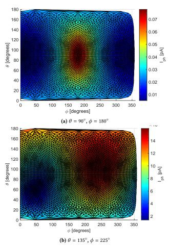
Figure 5: Unfolded (2D) photocurrent map for the spherical camera, when illuminated from a) the side, and b) at an angle.
